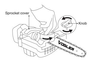
Loosen the screw by turning counterclockwise the knob until the sprocket cover comes off. Remove the sprocket cover. Remove the saw chain and guide bar from the tool.
