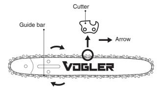
Fit in one end of the saw chain on the top of the guide bar. At this time, fit the saw chain as shown in the figure because it rotates in the direction of the arrow. Sprocket cover
