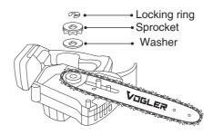
Always fit a new locking ring when replacing the sprocket.
