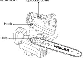
Insert the hook of the sprocket cover into the hole in the tool and then place the sprocket cover on the tool.
