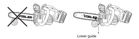
Bring the lower guide into contact with the branch to be cut before switching it on. Cutting without bringing the lower guide into contact
