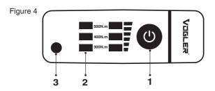
Indicator (2) displays the torque level ranging from 300N.m to 500N.m. Adjust the force by pressing trigger switch (1). Use button number (3) to change the device's direction.
