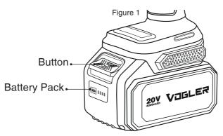
When removing the battery pack, press the button located on the front side of the battery pack and pull it out of the tool at the same time. When installing it, ensure the tongue spring on the battery pack aligns with the groove on the cover. Then, push and slide it into place until fully inserted, locking it with a click. If the red indicator on the upper side of the button is still visible after insertion, it indicates that the battery pack is not fully locked.
